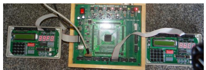
Fig -3: Real time implementation using FPGA and 7 segment LED.
